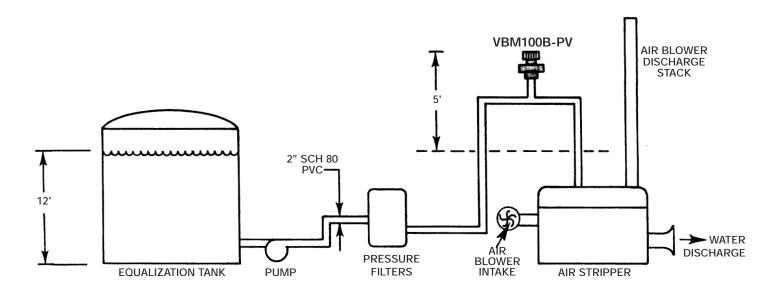
VBM Series Vacuum Breaker complements a ground water remediation process by elimination of siphoning. The remediation process, illustrated on the diagram, begins with chemical treatment in the equalization tank. This tank serves to balance effluent in a batch type process. Prior to installation of the VBM, siphoning would occur
